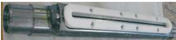
Back-flushing canal made of stainless
