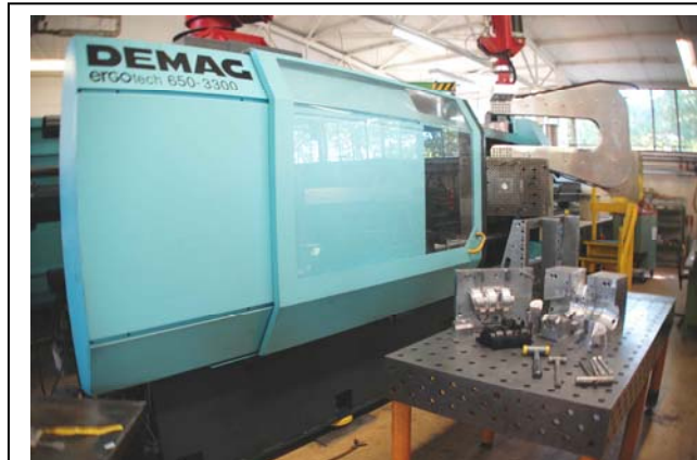
Typical production arrangement showing robot arm and assembly/demold platform
